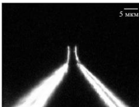
Рисунок 8.17 Нанопинцет (Korea Advanced Institute of Science and Technology)
